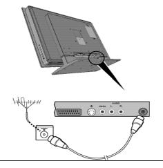
**4.** Connect the outside aerial or cable network to the socket at the back of the TV set.
